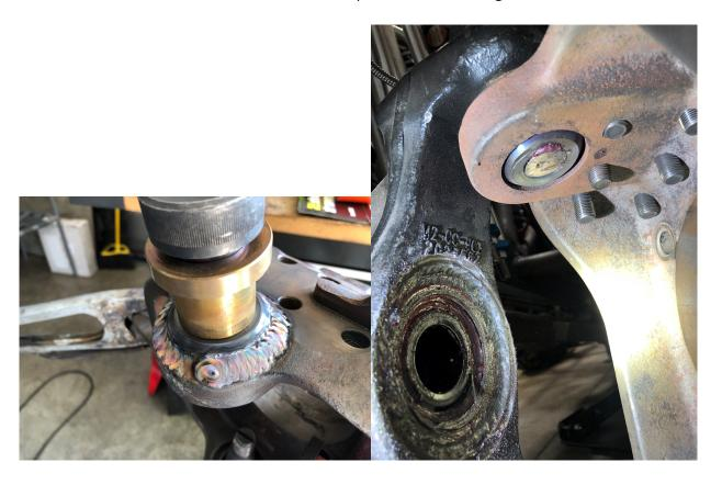
• Grind the lower balljoint until about 3/16" of thread is left.
