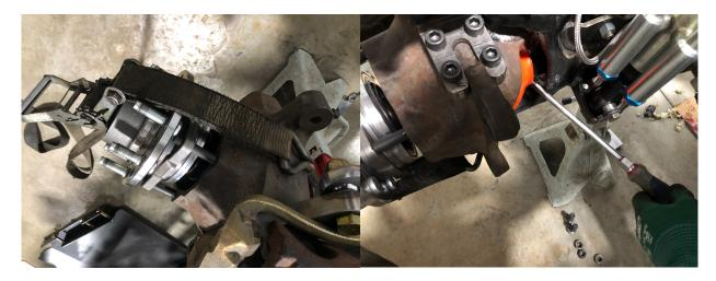
• Rotate knuckle all the way forward then back to access unit bearing nuts.
