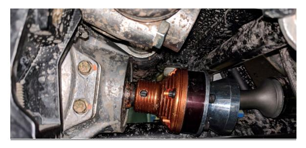
**Step 3** Once installed, remove the rear prop shaft slip flange along with the gasket and place them onto the protruding spline of the slip spline tube stub inside the carrier bearing. Install of the center CV and slip may vary between XP Turbo and XP 1000 machines.
