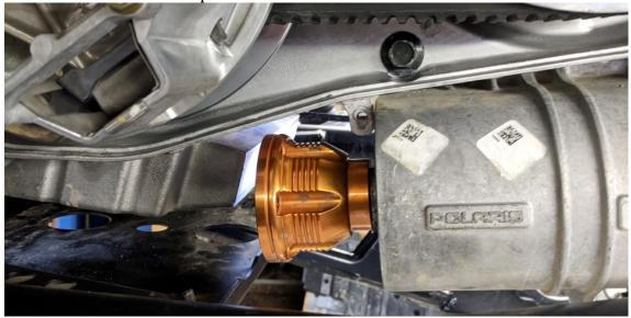
**Step 6** Install the rear prop shaft from the rear on the driver side of the vehicle. This will be done inbetween the belt box and the chassis.
