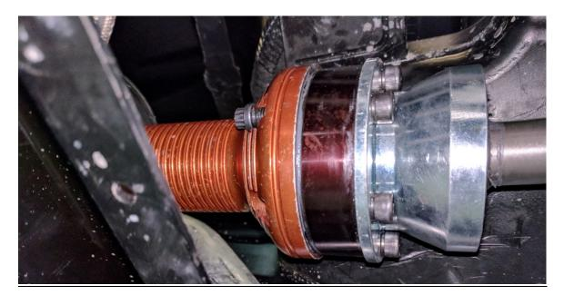
**Step 8** Mate the rear prop shaft with the flange connected to the rear output shaft then bolt together. Torque supplied bolts to 16 ft-lbs.
