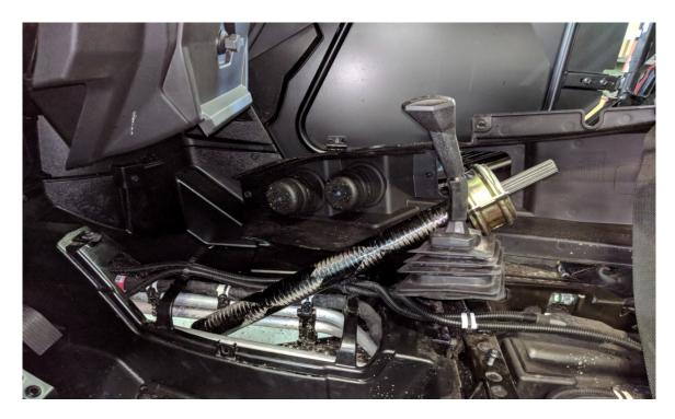
**Step 2** Slide the front prop shaft forward until it engages onto the input shaft of the front differential. <u>DO</u> NOT INSTALL ROLL PIN YET
