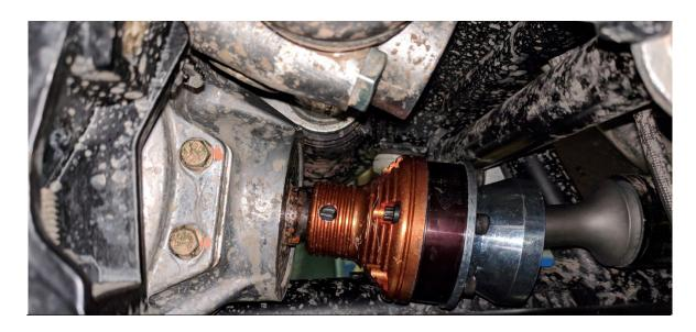
**Step 3** Once in place, you may begin to install the carrier bearing housing back onto the shaft and mock in place.
