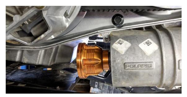
**Step 6** Install the rear prop shaft from the rear on the driver side of the RZR and align the splines onto the front half of the prop shaft. This will be done in-between the belt box and the chassis. This will be a tight fit, even with the motor mount disconnected.
